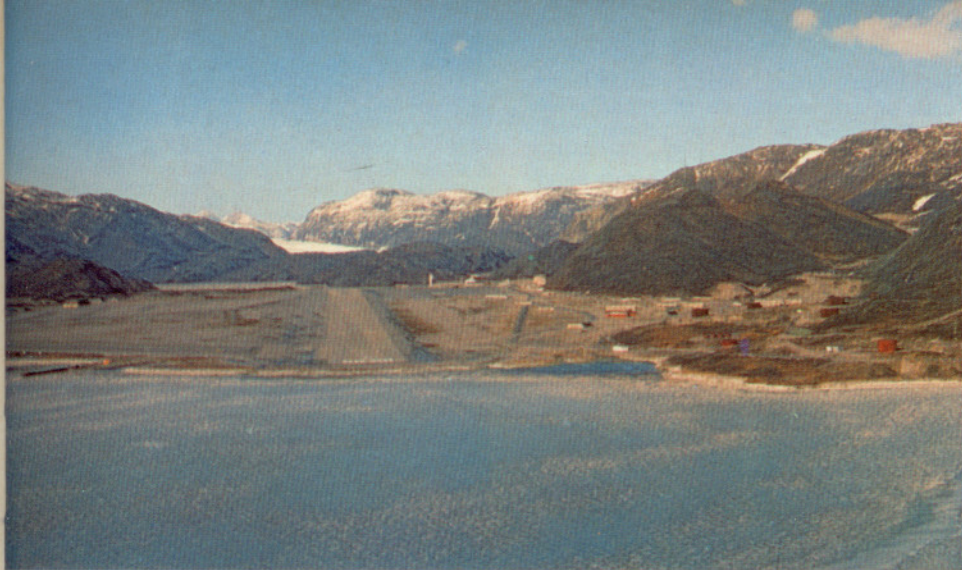
Rounding the final fjord, the pilot finds himself on short final to Narsarssuak Airport. Approach end of 6,500-foot runway is 10 feet above sea level. The other end is 136 ASL.
